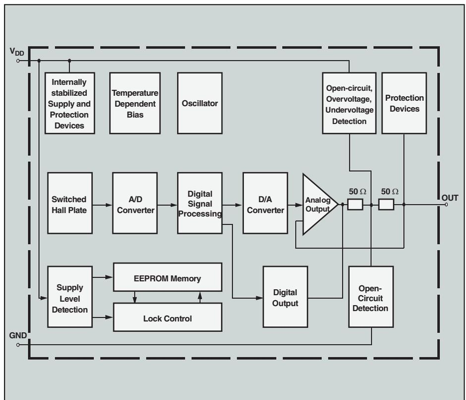
Fig. 2: Block diagram of the HAC 830
