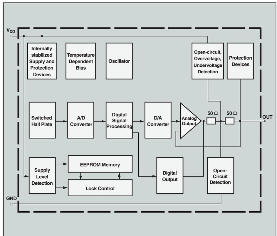
Fig. 2: Block diagram of the HAL 83x
