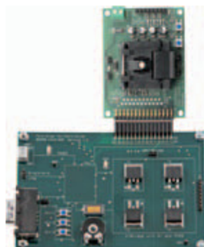
SPAB with HVC card for brush-type DC motor control
